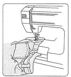
bar tacking to reinforce pockets, belt loops and waistline on readymade or homemade garments to avoid fabric bunching around the needle.
